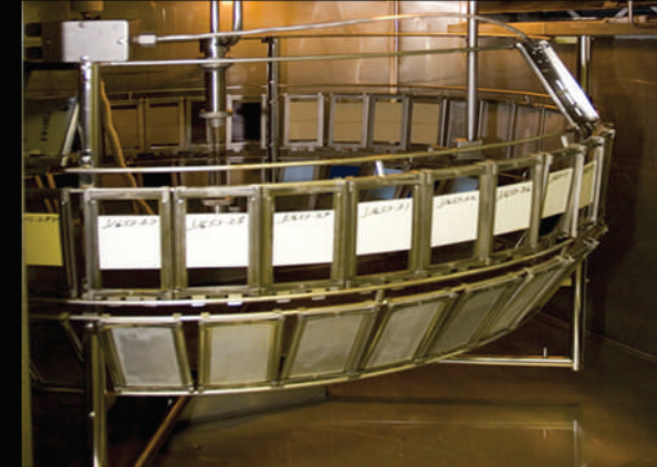
TEX-COTE® COOLWALL® coatings undergo extensive testing for fade resistance. Every 1000 hours of testing is equivalent to approximately two years of exterior exposure.
